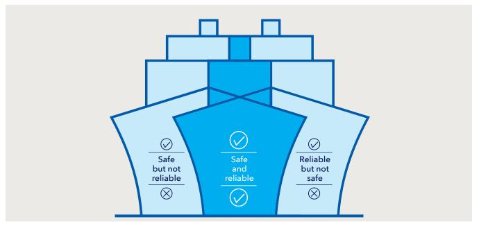
Figure 5-1: Safety and reliability in complex software-intensive systems, showing that information about reliability alone cannot lead to conclusions about the safety of a system. Concept reproduced from DNV GL's White Paper - Safety Assurance of Complex Systems.
