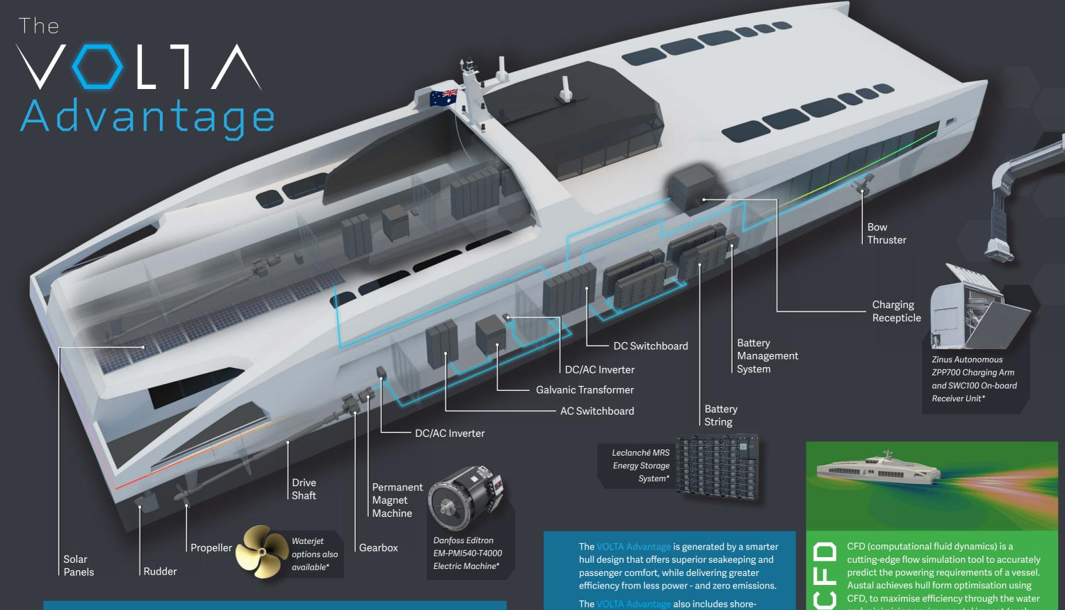
Austal's VOLTA series is the future of commercial commuter ferry operations, with vessels that are better for the environment, better for passengers and better for operators.
