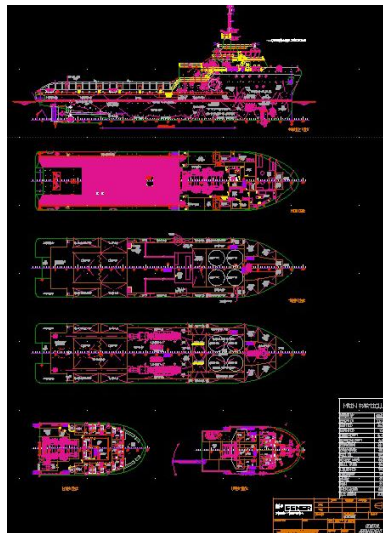
Figure 3: General Arrangement of a ship using a CAD System
