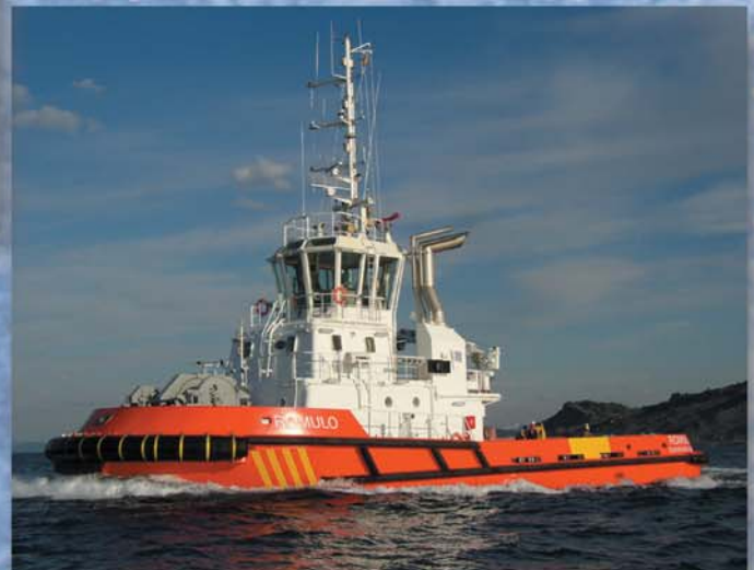
"Romulo" and "Remo" , 83t Bollard Pull ASD tugs for Repasa
