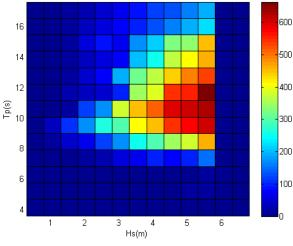
Figure 4: Power matrix of the device (kW)
