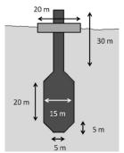
Figure 1: Two body heaving converter analyzed
