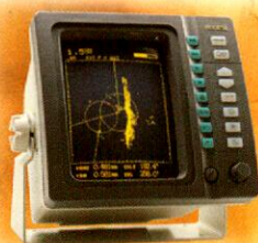
RA770, 10", 4kW, Radome 2 pies, 36 M.N. RA771, 10", 4 kW, Abierta de 3 ó 4 pies, 46 M.N.
